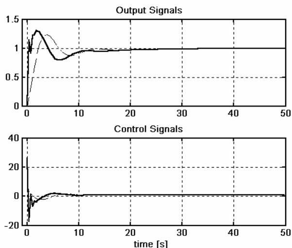
Fig. 7. The output and control signals of the analog (the dashed line) and the optimized ACS
