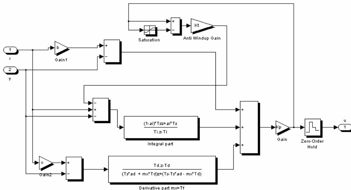
Fig. 1. Scheme of the universal digital PID controller with implemented anti-windup mechanism
