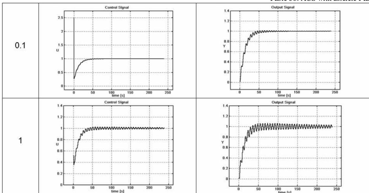
Table 6a. The tuned ACS with analog PID controller
