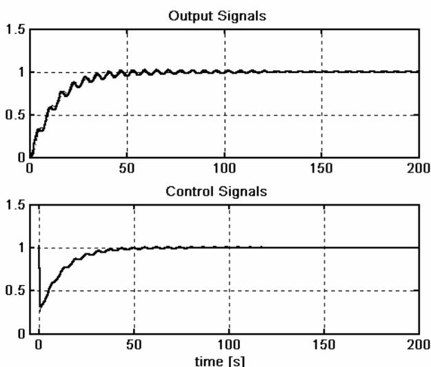
Fig. 5.  $y$  and  $u$  of the analog (the dotted line) and the optimized ACS
