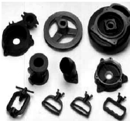
Figure 7. Pieces casted in shapes made through Rapid Tooling
