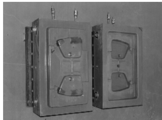
Figure 3. Metallic mould made through SLS
