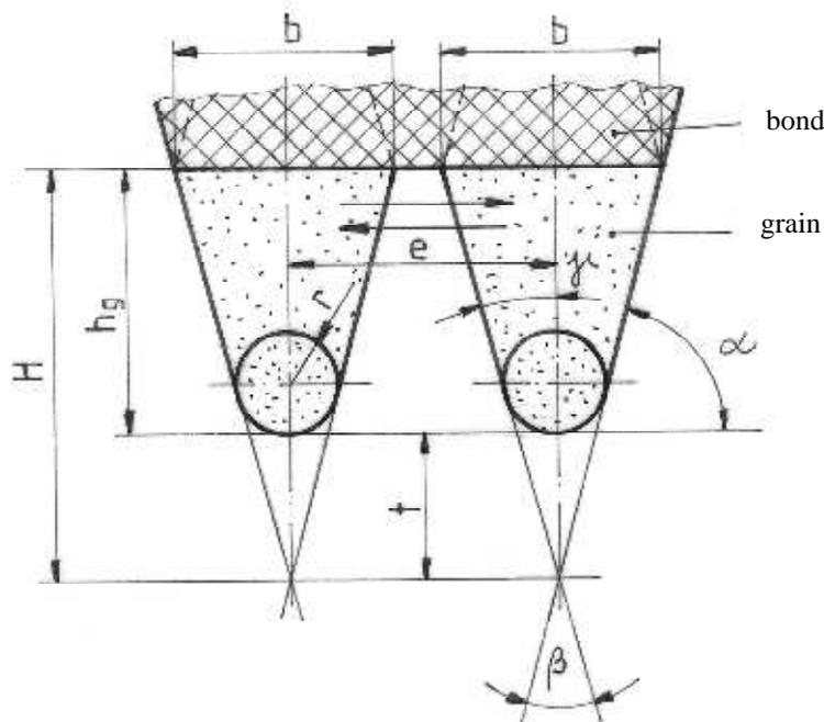
Figure 2. The spherical model of grain at machining with abrasives
