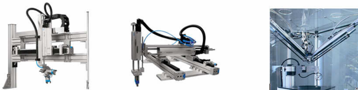
Figure 2. Utilisation of pneumatic drives in robot construction
