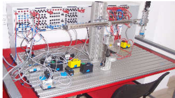
Figure 4. Electro-pneumatic manipulator system with gripper
