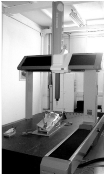
Figure 1. General view of the Coordinate Measuring Machine Brown & Sharpe Scirocco- MP, used for verification of the parts (with permission)
