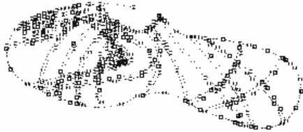
Figure 6. Drawing after FITARC command – over 70% less points
