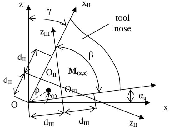
Figure3. The coordinates system on the tool, for temperature determination
