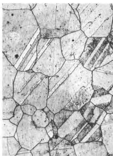
Figura 1. Oțel austenitic 2MoNiCr175 (atac cu acid cromic) Figure 1. Austenitic steel 2MoNiCr175 (chrome acid attack)
