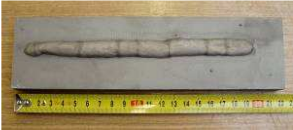
Figure 1. Weld bead onto steel
