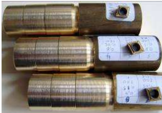
Figure 2. Machined specimens and inserts
