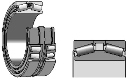
Figure 1. Conic roller radial – axial bearing
