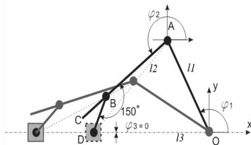
Figure 8. Kinematic diagram of the flexible bar mechanism
