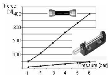
Figure 4. Forces developed by a pneumatic muscle and a pneumatic cylinder
