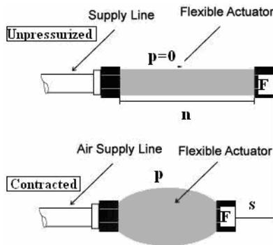
Figure 2. Working principle of a pneumatic muscle
