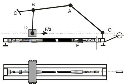
Figure 6. Operating principle of the isokinetic equipment
