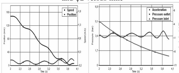
Figure 12. Variation of the muscle position, speed and acceleration versus time
