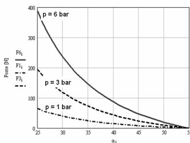
Figure 3. Force versus enveloping angle and working pressure
