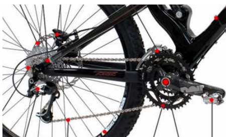
Figura 12. Transmisia cu lanț a unei biciclete moderne Figure 12. Sprocket chain gearing of a modern bicycle
