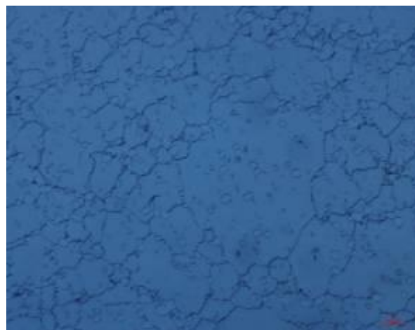
Figure 2. Rp5 high speed steel hardened (with heating in salt baths) Nital attack; 1000:1
