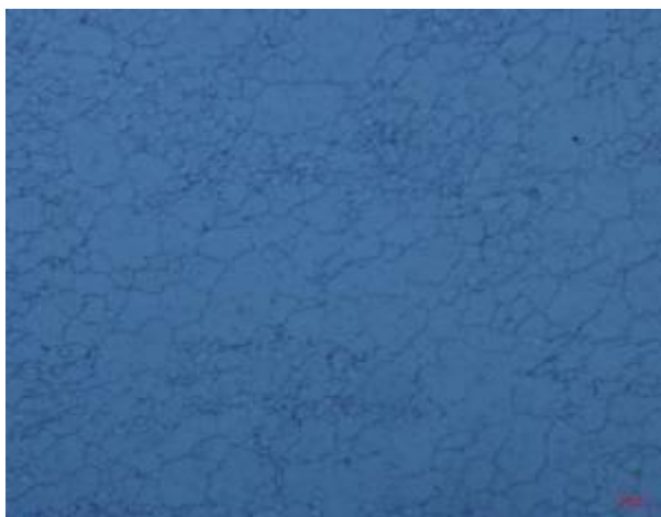
Figure 1. Rp5 high speed steel hardened (with heating in salt baths) Nital attack; 500:1
