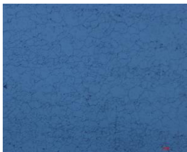
Figure 7. Rp5 high speed steel hardened in vacuum Nital attack; 500:1
