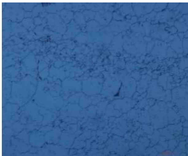
Figure 5. Rp5 high speed steel, superheated quench (1250 °C) Nital attack; 500:1
