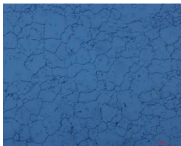
Figure 8. Rp5 high speed steel hardened in vacuum Nital attack; 1000:1
