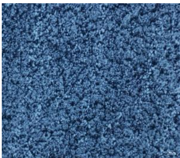
Figure 9. Rp5 high speed steel hardened and tempered in vacuum Nital attack; 500:1
