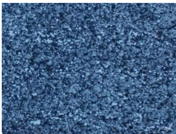
Figure 3. Rp5 high speed steel hardened (with heating in salt baths) tempered at atmospheric pressure Nital attack; 500:1
