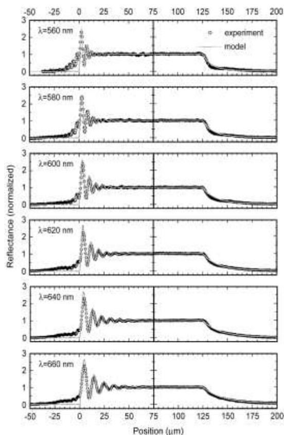
Figure 5. SPR response to a dielectric step at several wavelengths. For each wavelength the light angle of incidence is set such that outside the strip (extending from 0 to 125  $\mu\text{m}$ ) the interrogating  $k_x$  is resonant with the surface plasmon wavevector. The surroundings of the strip has dielectric constant  $\epsilon_3 = 1$  [13]
