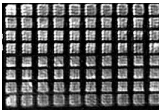
Figure 6. Typical image obtained with an SPR imaging sensor with a polarization control. Bright rectangles correspond to areas of an SPR chip ( $300 \times 300 \text{ mm}$ ) covered with a monolayer of albumin molecules formed on the surface of gold by microspotting [13]
