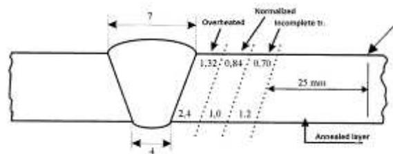
Figure 11. Welded Sub-seam width  $\Phi 168.3 \times 8$ .
