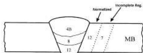
Figure 12. Metallographic grain size welded pipe  $\Phi 168.3 \times 8$  - OLT 35
