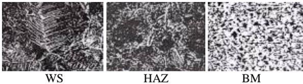
Figure 8. Metallographic structure of manually welded seam with coated electrode, the pipe  $\Phi 108 \times 4$  OLT 45 (240:1)
