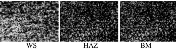
Figure 9. Metallographic structure of the welded seam in a gas protective environment (MAG with “very short arc spray”) pipe  $\Phi 108 \times 4$  OLT 45 (240:1)
