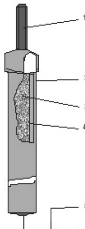
Figure 5. Tubular electrode used for hardfacing
