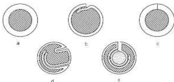
Figure 6. Types of tubular electrode sealing profiles to welded pipe, b-pipe with rolling, pipe rolling c-butt Folding d-bore, double-barrelled e-Folding
