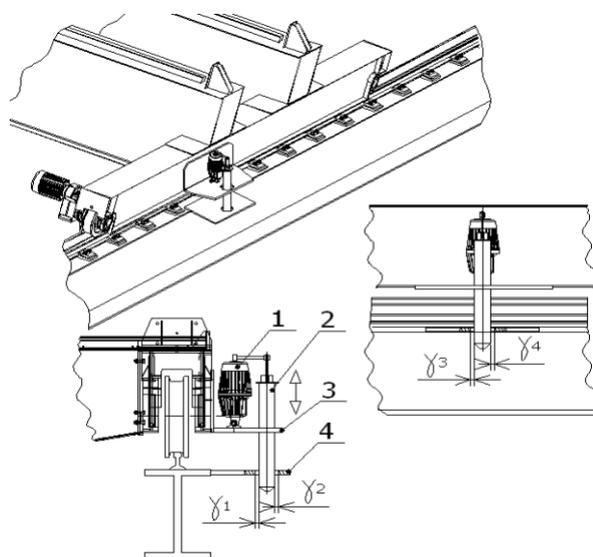
Figure 12. Locking mechanisms of crane bridge
