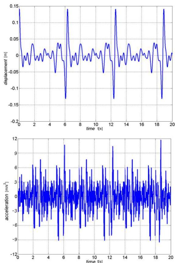
Figure 3. Input seismogram and accelerogram
