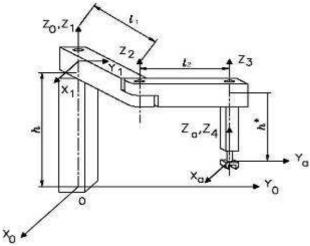
Figure 2. SCARA manipulator
