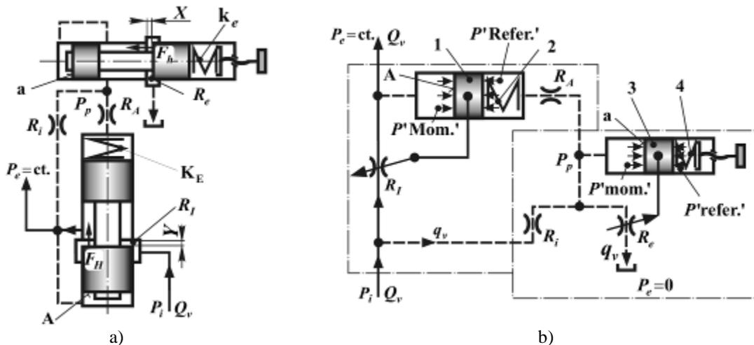
Figure 3. Piloted pressure reducing valve
