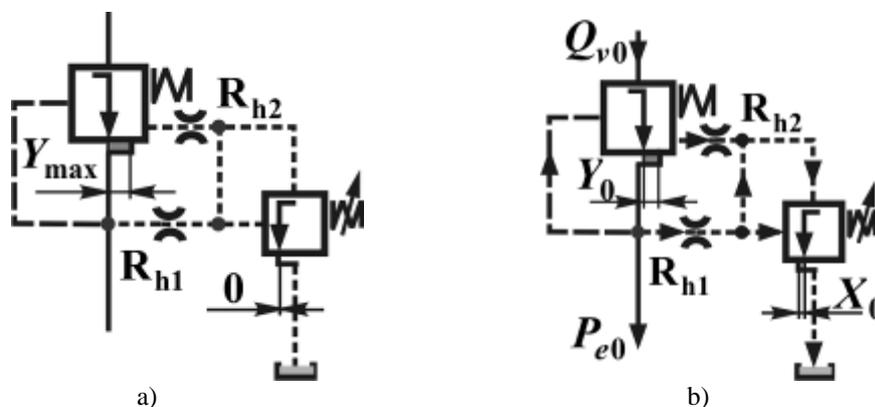
Figure 6. Piloted reducing valve
