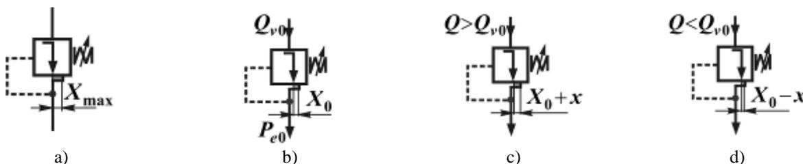
Figure 5 Normally open valves working phases
