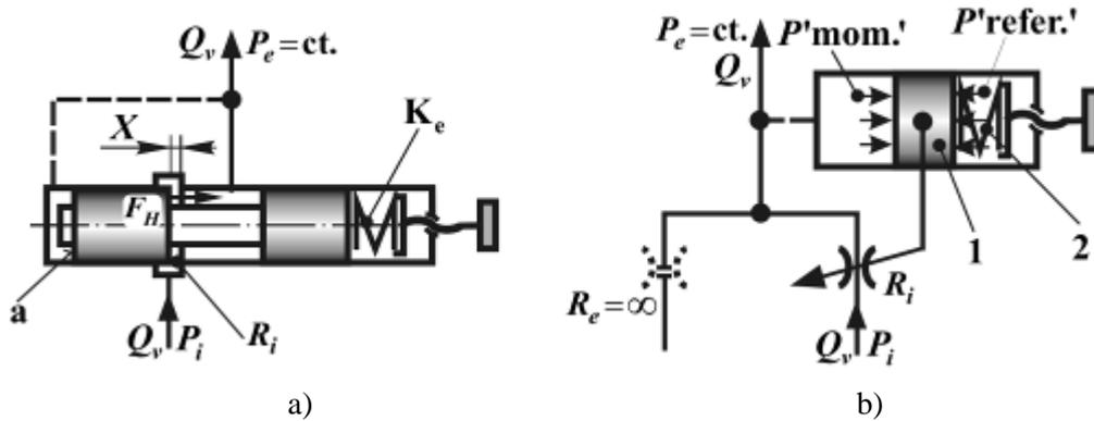
Figure 2. Direct pressure reducing valve
