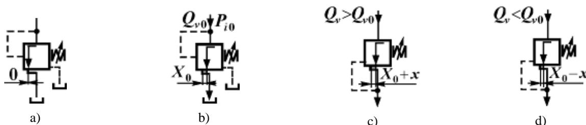
Figure 4. Normally closed valves working phases
