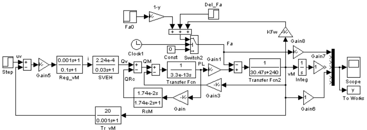
Figure 4. Simulation diagram (system with MHL + RcM)
