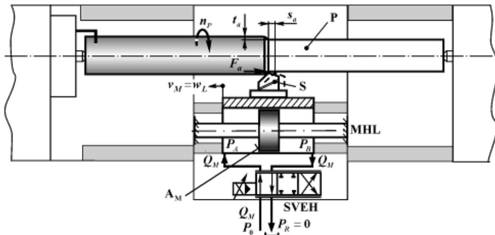
Figure 1. Electro-hydraulic system for the feed speed
