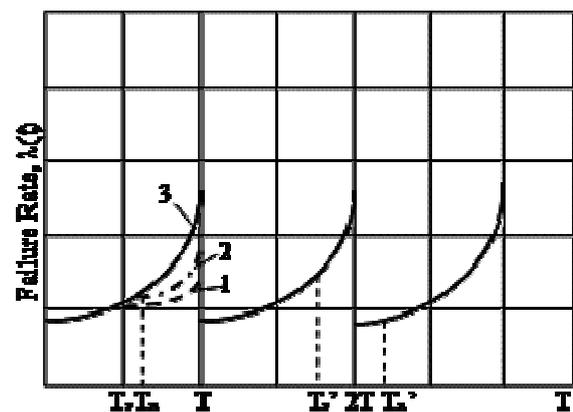
Figure 1. Failure rate curves, presenting three types of repair models: “as-good-as-new” (1); “as-good-as-old” (2); continuous aging (3).
