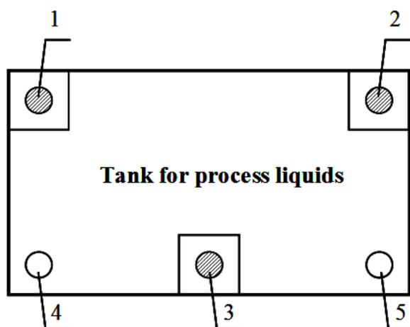
Figure 2. Tank heating system with 3 main and 2 spare burners of a “hot sticks” type.
