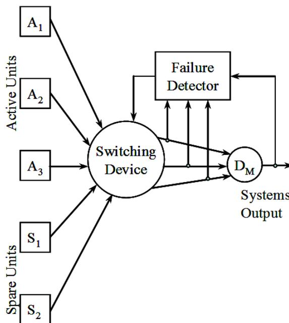
Figure 3. Reliability configuration of a TRM tank heating system
