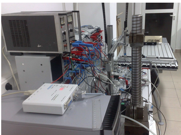
Figure 1 Experimental stand for the study of pneumatic muscles
