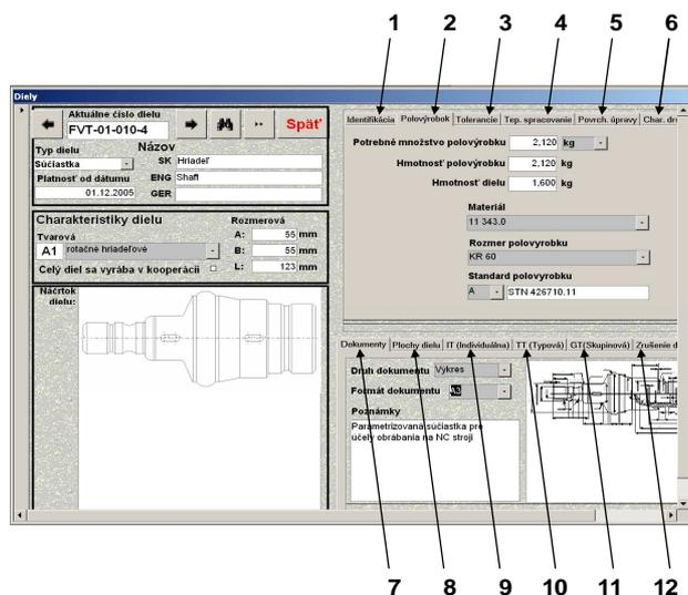
Figure 2. Interface for definition of properties and characteristics of production segment (part, subassembly ... final product) [4]
