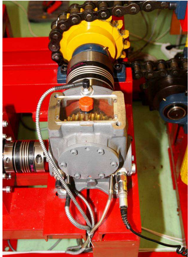
Figure 2. The placing of the sensors on the surface of worm gearboxes
