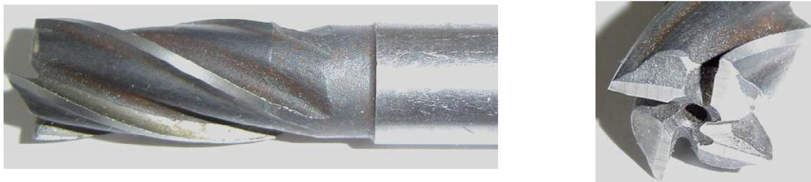
Figure 2. End-milling cutter used
