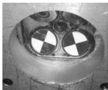
Figure 4. Markers positioned on valve head
