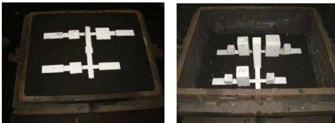
Figura 6. Execuția formei Figure 6. Manufacturing of the mould
