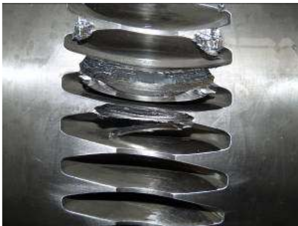
b) Damage over the worm gear
