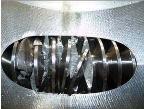
a) Damage over the worm
