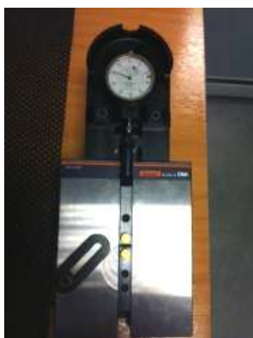
Figura 6. Ceas comparator Diatec asamblat cu suport DM1 Figure 6. Diatec caliper assembled with DM1 support
