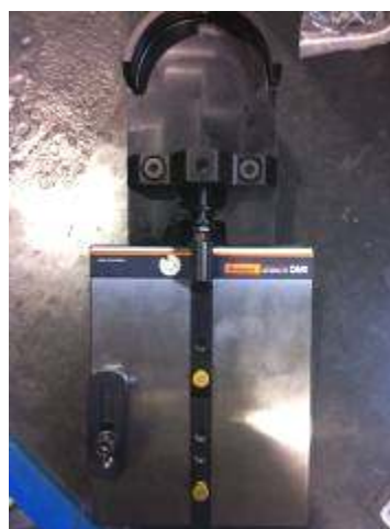
Figura 6. Ceas comparator Diatec asamblat cu suport DM1 Figure 6. Diatec caliper assembled with DM1 support
