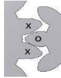
Figure 5. Marking of gear drives with N_A > 1
