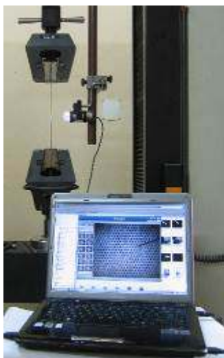
Figure 6. Experimental set for simultaneous registration of image-deformation changes
