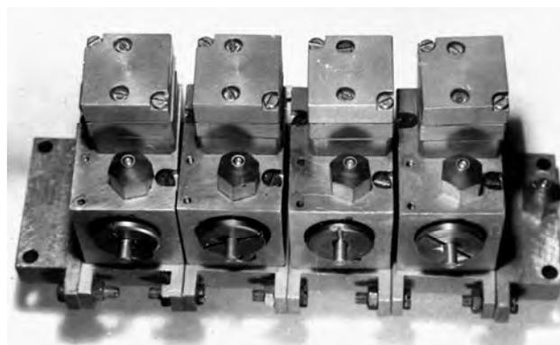
Figure 5. SMB with integrated cells
