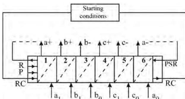
Figure 8. Cyclo-diagram of a successive sequential cycle
