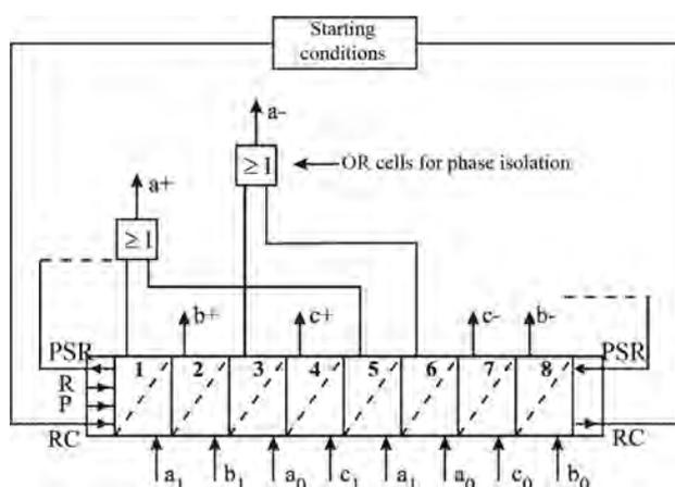
Figure 9. Cyclo-diagram of a repetitive sequential cycle
