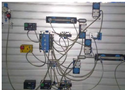
Figure 7. STEPPER circuit as pneumatic PLC
