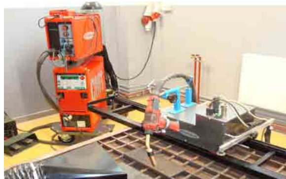
Figure 2. FRONIUS installation GMAW-CMT
