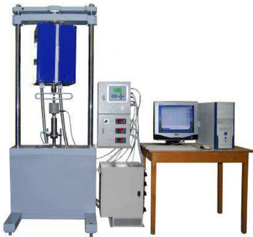
Figure 2. A stand for testing materials at elevated temperatures
