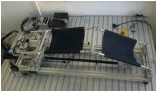
Figure 1. A human recovery apparatus motorized with a pneumatic artificial muscle of type MAS-20-750N-AAMC-O-ER-BG (Festo AG & CO)
