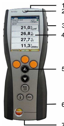
Figure 2. Control Unit: 1 - IrDA interface; 2 - Switch On / Off; 3 - Magnetic holder (on rear); 4 – Display; 5 – Keyboard; 6 - Contact bar for meas. box (on rear); 7 - Interfaces: USB 2.0, charger, Testo Data bus
