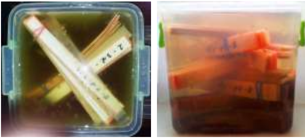
Figure 3. Specimens immersed in 5 % NaCl aqueous solution
