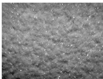
Figure 4. Granulometric structure of aluminium oxide after presintering
