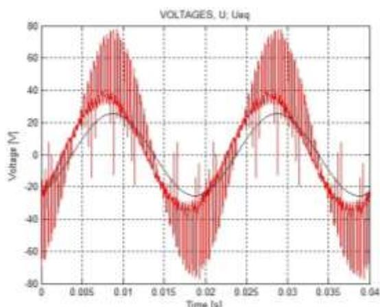
Figure 5. The load voltage (1) measured values – the thick plot, and (2) the estimated values – the thin plot. Duty cycle  $a = 0.6875$
