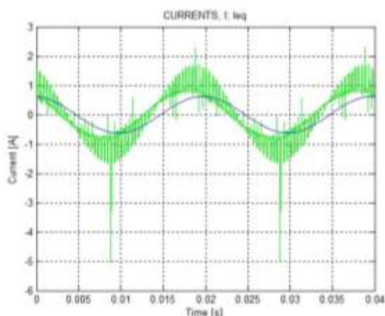
Figure 6. The plot of the load current (1) measured values – the thick plot, and (2) estimated values – the thin plot. Duty cycle  $a = 0.6875$
