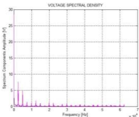
Figure 7. The amplitude spectral density of the load voltage. Duty cycle  $a = 0.6875$
