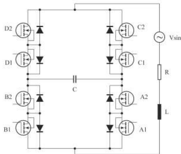
Figure 2. The electrical diagram of the proposed electronically switched capacitor, [2]
