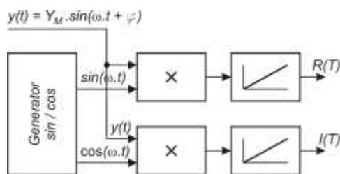
Figure 1. The schematic of the frequency analyzer principle
