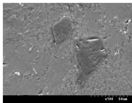
Figure 1. SEM image. Showing SiC particles embedded as well as the areas of quasi dispersion of the graphite in the SiC p zones
