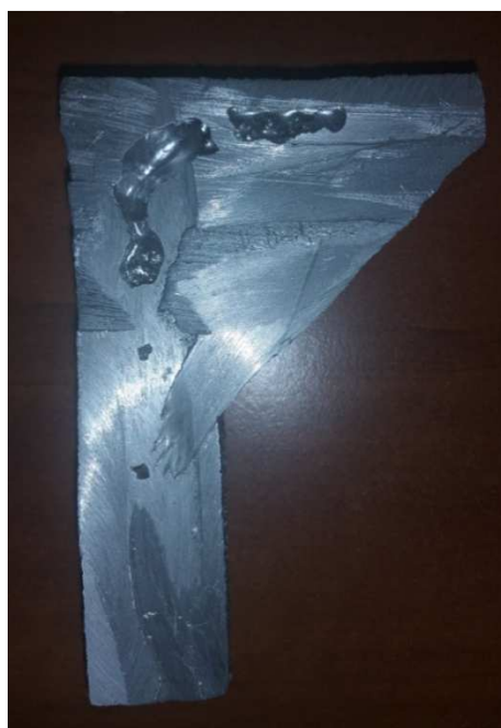
Fig. 19. Shrinkage location in experimental casting
