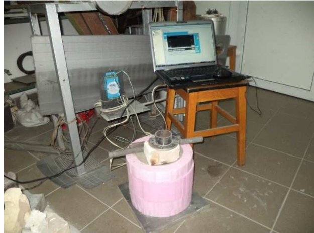
d. temperature measuring and recording installation
