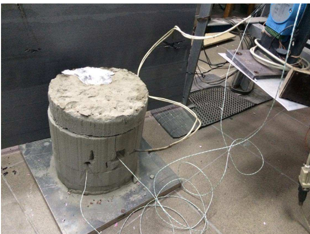
e. solidification of the cast alloy
