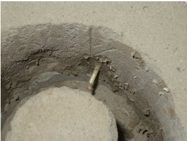
c. position of "B" thermocouple
