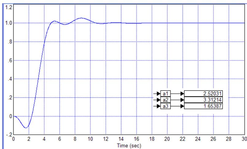
Fig. 5. Resulting transient process in the structure of figure 3 with the weight coefficient  $k = 0$ , i.e. with cost function (5)
