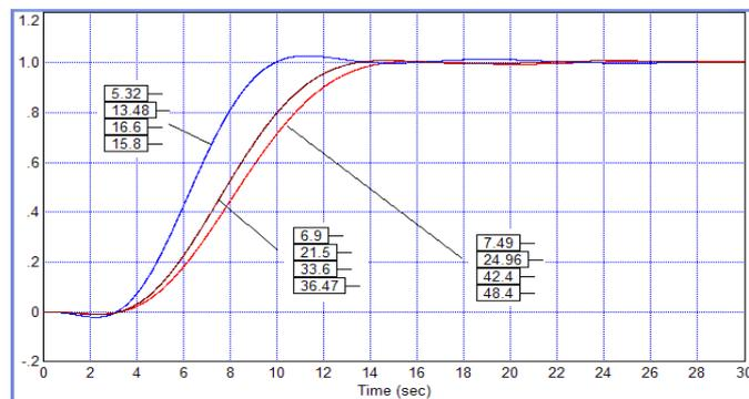
Fig. 12. Resulting transient process in the structure of figure 11, with a weight factor  $k = 10$  (blue line),  $k = 75$  (black line) and  $k = 100$  (red line); at weight factors 10 and 50 the result are almost the same (lines are merged)
