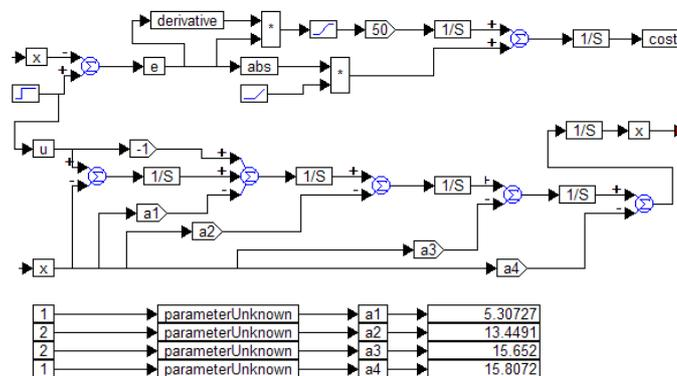
Fig. 11. Structure for optimization of the fifth-order filter according the cost function (6), (7)
