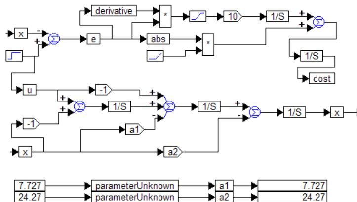
Fig. 8. Structure for optimization of the fourth-order filter according the cost function (6), (7)
