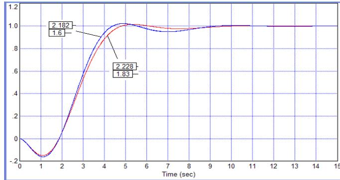
Fig. 10. Resulting transient process in the structure of figure 8 according the cost function (4) (blue line) and the cost function (5) (red line)
