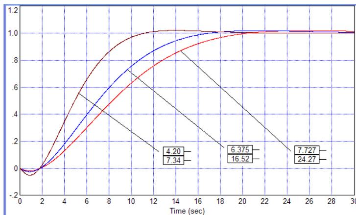
Fig. 9. Resulting transient process in the structure of figure 8 with a weight factor  $k = 10$  (black line),  $k = 20$  (blue line) and  $k = 100$  (red line)
