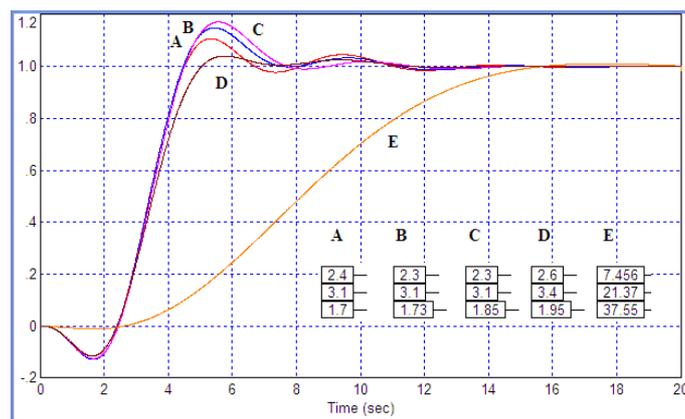
Fig. 2. Transients in filters with different characteristic polynomials from Table 3
