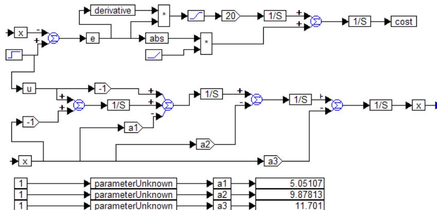
Fig. 3. Structure for optimizing of the fourth-order filter according the cost function (6), (7)
