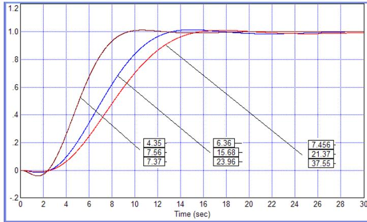
Fig. 7. Resulting transient process in the structure of figure 3 with a weight factor  $k = 10$  (black line),  $k = 20$  (blue line) and  $k = 100$  (red line)
