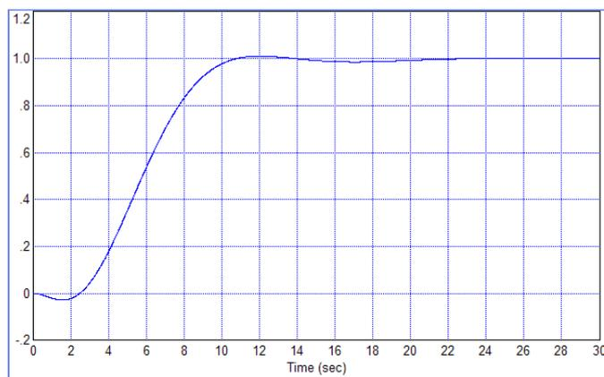
Fig. 4. Resulting transient process in the structure of figure 3 with the weight coefficient  $k = 20$
