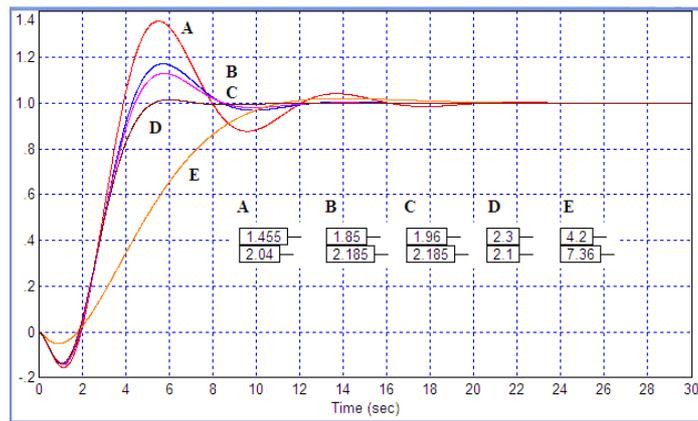
Fig. 1. Transients in filters with different characteristic polynomials coefficients from Table 2
