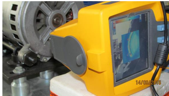
Fig. 2. The thermal camera location with respect to the electrical motor
