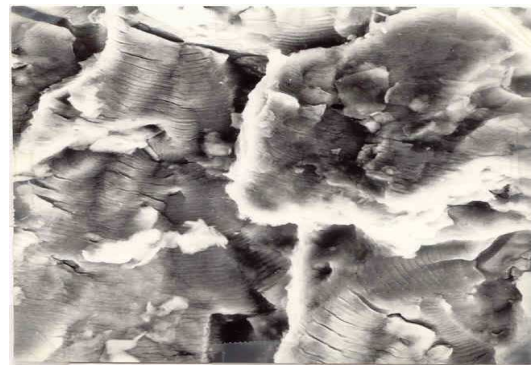
d. Fracture surface detail. The direction of crack growth at the level of material grains is evident (x3000)
