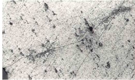
b. Metallographic micrograph showing different manganese compounds developed within the immediate area of the fatigue crack (x400)
