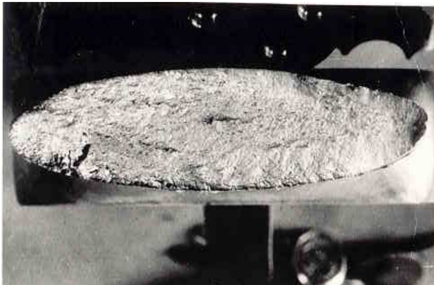
Fig. 11. Cross section of the propeller blade subjected to fatigue
