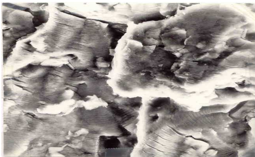
Fig. 12. Fracture surface detail (x3000)
