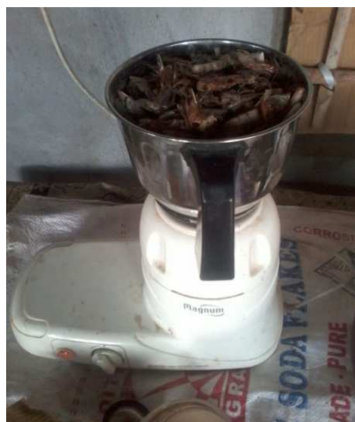
Fig. 3. Blending of dried prawn shells
