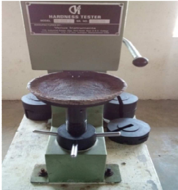
Fig. 9. Conducting hardness test on the test piece
