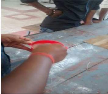
Fig. 6. Mixing of the resin and hardener
