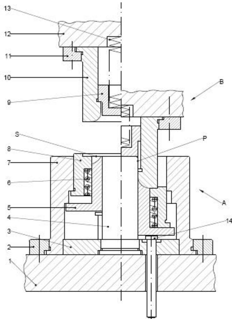
Fig. 3. Combined blank holding deep drawing die
